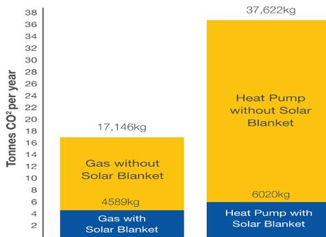
Graph is based on data and figures from "pool heat" simulation program. Pool in Sydney heated to 28°C year round. CO<sup>2</sup> Coefficient 1.381kg/kwh - electricity 0.055 kg/Mj - gas
